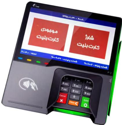
In some of Tehran's metro stations the PX7 was installed as a stand-alone unit, while in others a peripheral printer box was connected to it.
